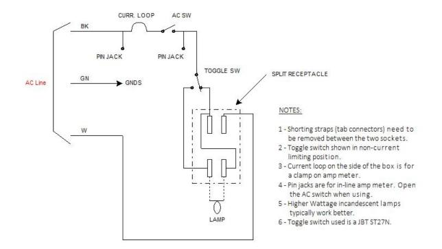
I would have liked to have added a fuse and pin jacks to measure the actual voltage applied to the device but the box was running out of space. There are some wire nuts (Marr connectors) used that also took up space in the box.
