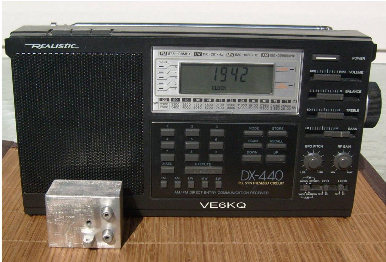
I now use it almost exclusively to monitor the 20 meter AM frequency, 14.286 MHz. There was a problem here also. When connected to a decent outside antenna it pretty much died due to front end overload from other signals. The receiver doesn't appear to have any front end selectivity. Turning down the the RF gain helped a little but not much.
