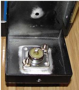
I checked the VSWR on 2 meters using a Bird 43 Wattmeter and after doing the conversion calculation it indicated about 1.5 to 1. Although the dummy load was not rated higher than 160 MHz, I checked it at 440 MHz. It was un-usable at this frequency.
