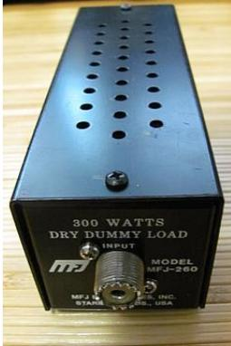
It looked in good shape but I checked the load resistor to see how close it was to 50  $\Omega$ . The measurement was taken at the SO-239 connector and it measured about 64  $\Omega$ .
