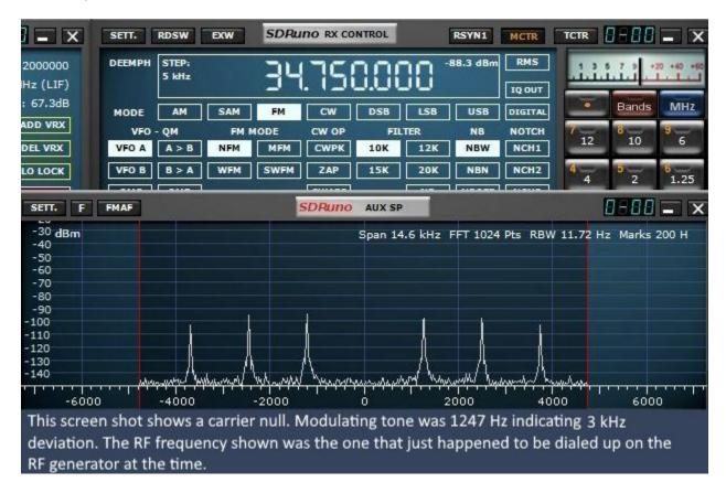
After the 3 kHz deviation was determined as shown above, the rf cable from the generator was transferred to the modulation monitor to verify that the meter reading was correct. The meter was on the 5 kHz scale. The meter accuracy was also checked at 5 kHz deviation and 1 kHz deviation on this scale. Some readings were also taken on the 10 kHz scale.
