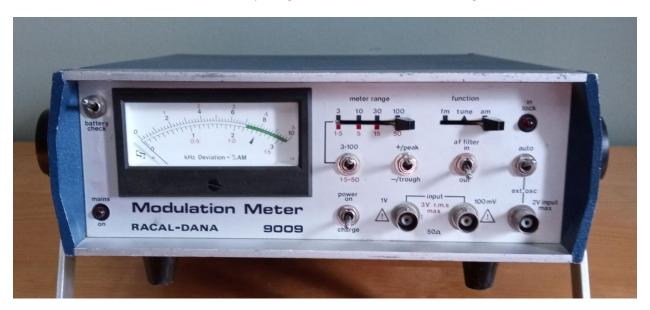
The basic operating frequencies were from 30 to 1500 MHz. This range could be extended somewhat by providing an external local oscillator signal. FM deviation measurements are up to 100 kHz. On the back of the unit there are 3 BNC connectors, they are <u>Audio Out</u>, <u>DC Out</u> that is a DC level proportional to the front panel meter reading and a 500 KHz <u>IF Out</u>. Both the audio output and the IF output are useful as described later.
