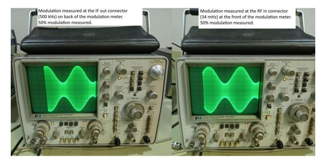
The above is a comparison between a 34 mHz signal at the input of the meter and the signal at the IF output.
