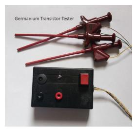
The tester tests for leakage and gain. I used clip on test probes as they were more convenient to use than a transistor socket. Many of the transistors to be tested were previously used and the leads were in various lengths and condition. To build the tester I used the parts I had on hand.
