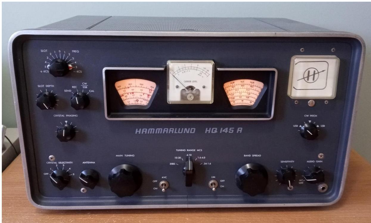
It is dual conversion above 10 MHz with IF's at 3035 and 455 KHz. It uses silicon diodes as a power rectifier. No product detector is included. It covers .54 MHz to 30 MHz in four bands plus the 20 meter amateur band has a special band spread position.
